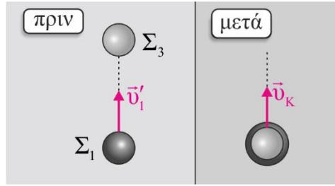
$$\vec{p}_{\text{πριν}} = \vec{p}_{\mu\epsilon\tau\alpha} \Rightarrow m \cdot v'_1 = 2m \cdot v_\kappa \Rightarrow v_\kappa = \frac{v'_1}{2 \cdot \sqrt{3}} \quad (3)$$
