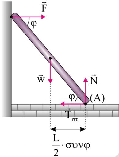
$$\sum \vec{F}_A = 0 \Rightarrow F \cdot L \cdot \eta \mu \varphi = w \cdot \frac{L}{2} \cdot \sigma v n \varphi \Rightarrow F = \frac{w}{2} \cdot \frac{\sigma v n \varphi}{\eta \mu \varphi} = \frac{w}{2 \cdot \varepsilon \varphi \varphi} \quad (1)$$
